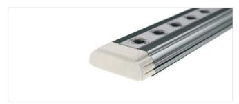
3. Attach the optional end cap (accessory) without OSRAM stamp in order to finish the module and to get the strain relief function for the connecting cables.
