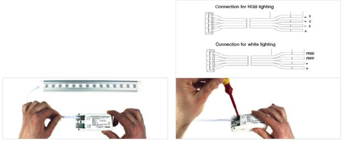
4. Connect the power supply cables (observe correct polarity) and close the cap.
