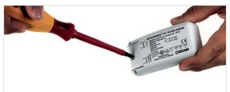
4. Open the cap of the control gear.
