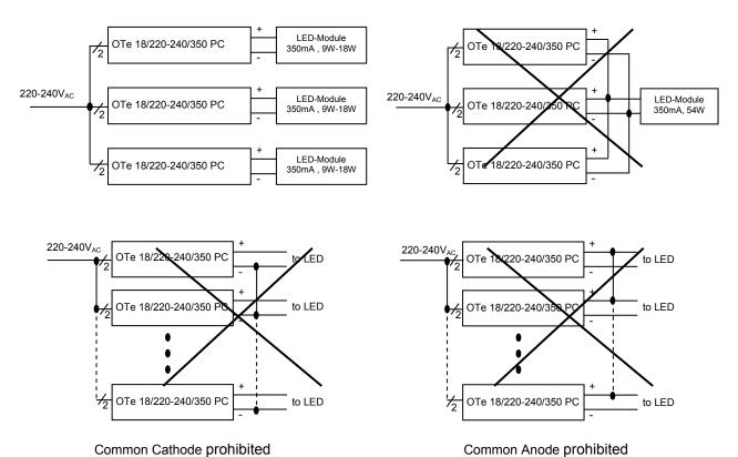
The installation of two or more OPTOTRONIC® OTe 18/220-240/350 PC Power Supplies with common "-" or "+" wiring by the intention to save wire to LED modules is prohibited, in order to avoid exceeding the maximum allowed system touch current levels on the accessible parts of the installation.
