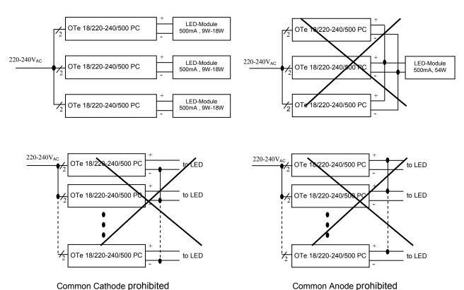
The installation of two or more OPTOTRONIC® OTe 18/220-240/500 PC Power Supplies with common "-" or "+" wiring by the intention to save wire to LED modules is prohibited, in order to avoid exceeding the maximum allowed system touch current levels on the accessible parts of the installation.
