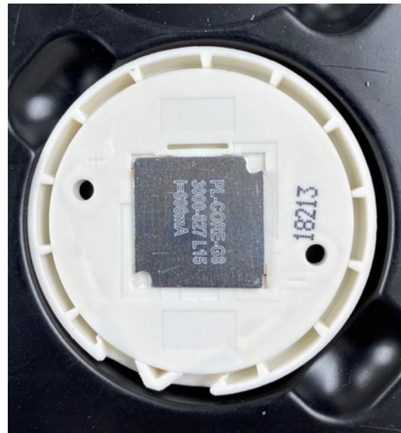
4 The connection between the LED COB and the holder is now established. The LED module is ready for installation.
