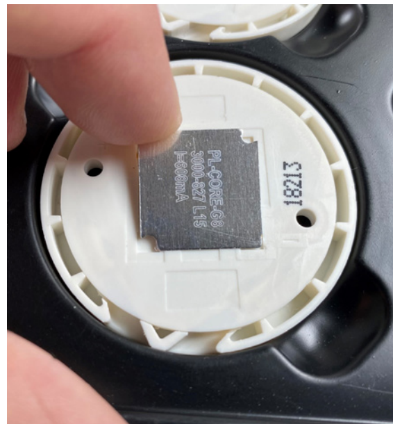
2 Turn the LED COB over and insert it into the back of the holder. Make sure that the polarity is correct.
