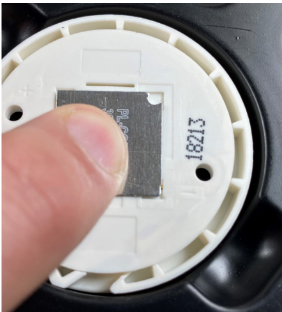
3 Now carefully press on the back of the LED COB until it clicks into place in the holder (at the notch on the side, as shown above).
