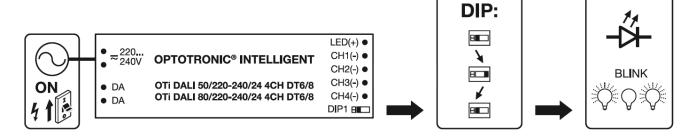
For instance, in order to reconfigure the driver for a new DT6 load configuration, after connecting or disconnecting new loads, move the dip-switch from ON to OFF, then from OFF to ON, during power-on or powering on after each operation.
