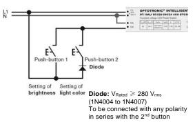
This driver supports single and double button Touch DIM operation. The 2<sup>nd</sup> button must be connected in parallel with the 1<sup>st</sup> by means of a diode. As per factory default configuration, the Touch DIM mode is auto-detected and stored through a Long Press of the 1<sup>st</sup> button; the operation is as follows:
