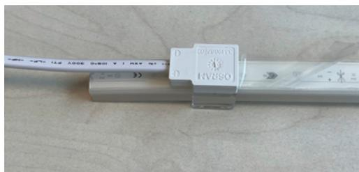
7. Ensure that the “hourglass” mark is still visible but not completely visible.
