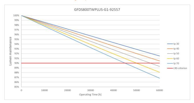
Note: Light flux varies with the temperature measured @Tc point; nominal values is given @Tc = Tp. Flux increases when Tc decreases.
