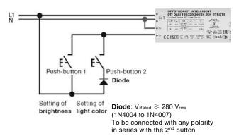
This driver supports single and double button Touch DIM operation. The 2<sup>nd</sup> button must be connected in parallel with the 1<sup>st</sup> by means of a diode.
