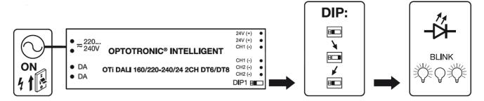
For instance, in order to reconfigure the driver for a new DT6 load configuration, after connecting or disconnecting new loads, move the dip-switch from ON to OFF, then from OFF to ON, during power-on or powering on after each operation.
