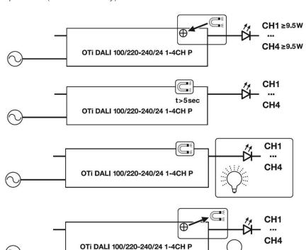
During normal operation, ensure each channel is loaded with at least 9.5W, then put the provided magnet on top of the sensor located where the  $\oplus$  symbol is printed on the driver.
