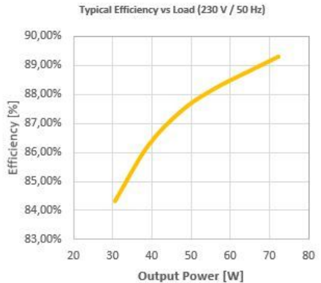
ETI DALI 75 LT2 L Typical Efficiency vs. Load
